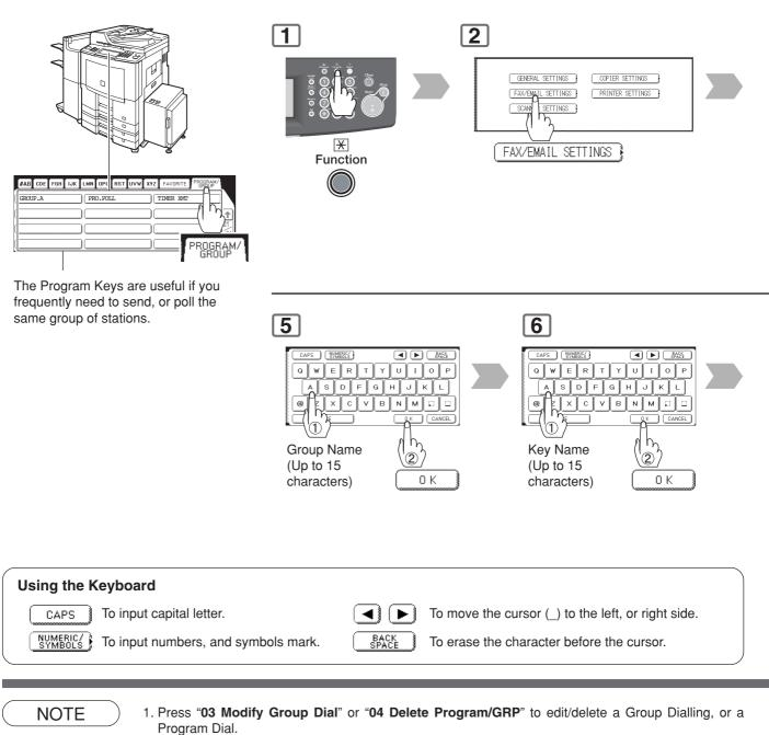
The Group Dialling, and Program Key cannot be changed or erased until the communication has finished. To change, or erase the settings, cancel the communication first by Edit File Mode. (See pages 120, 122)
